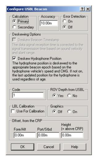
The *Accuracy* is the critical setting. This is generally between 7-15m, depending upon the performance of the USBL system. The lower the value, the greater the influence of the USBL data in the Kalman Filter. The higher the value, the less the influence of the USBL data in the Kalman Filter.
