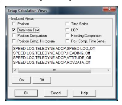
Select the *Data Item Text* checkbox, highlight the SPEED LOG item and then click the *On* button. Exit with *OK*. The speed log data can then be monitored in the Calculations window, as shown below.
